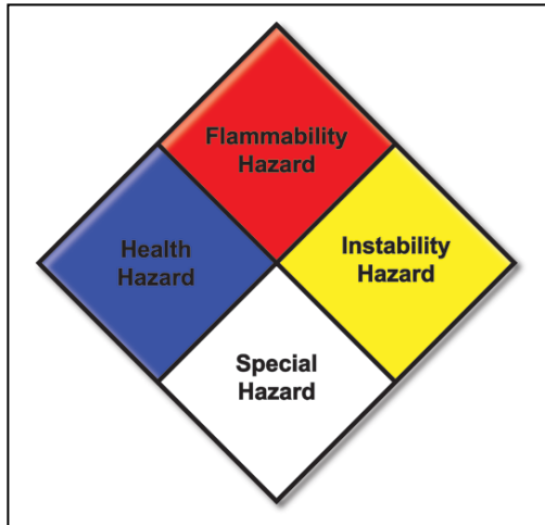
Figure 2: National Fire Protection Rating System (NFPR)
